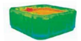
Standard hot tub without full-foam insulation.
