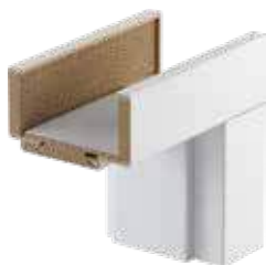
door frame profile - architrave 80 mm for door height 200 - architrave 100 mm for door height 220
