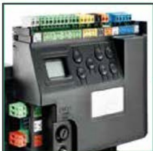
Programming interface and extractible terminal blocks
